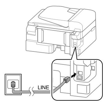
**Note:** If you have a DSL or ISDN connection, you must connect the appropriate DSL filter, or ISDN terminal adapter or router to the wall jack to be able to use the line for faxing or voice calls using your product. Contact your DSL or ISDN provider for the necessary equipment.
